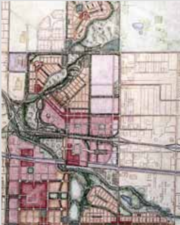
FIGURE 5-55 The community plan, shown on the left, is organized around two day lighted creeks, formerly buried under airport runways, and a series of secondary conveyances which provide recreational open space within neighborhoods. The image on the right illustrates one of the multi-functional creek corridors. Consolidated stormwater treatment areas and surface conveyances define more traditional park recreation and play areas. Courtesy of Stapleton Redevelopment Foundation.
